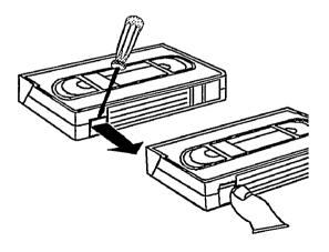
So that you don't accidentally delete an important recording, you can remove the special tab (erase protection) on the narrow side of the cassette with a screwdriver.
